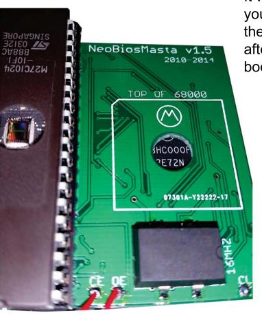
It will have a tight fit, but for added strength, you can add a small amount of hot glue to the hole on top. I recommend doing this after you have confirmed your system is booting your new bios.
