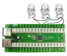
The Mini-PAC and I-PAC UIO use a supplied wiring harness. The harness comes in two sections. There is a "daisy-chain" ground harness and a 32-way switch harness.
