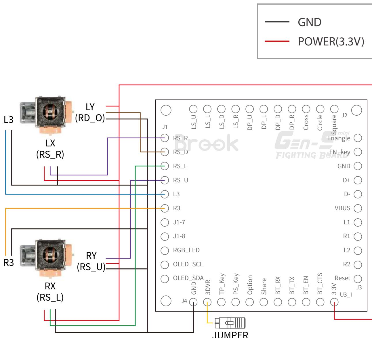
\*If a digital-analog joystick is installed, the stick will not be able to switch between RS/LS modes.
