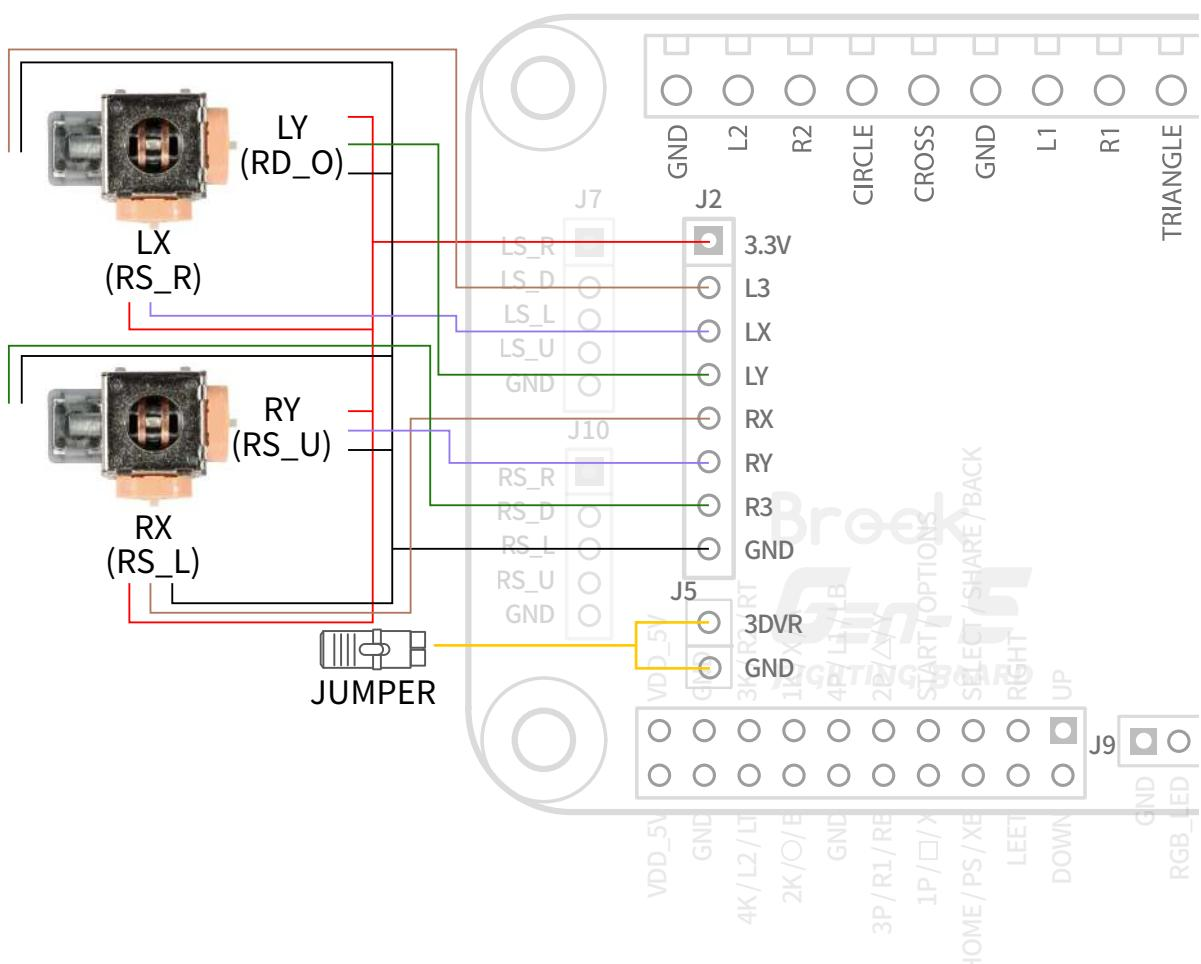
\*If a digital-analog joystick is installed, the stick will not be able to switch between RS/LS modes.
