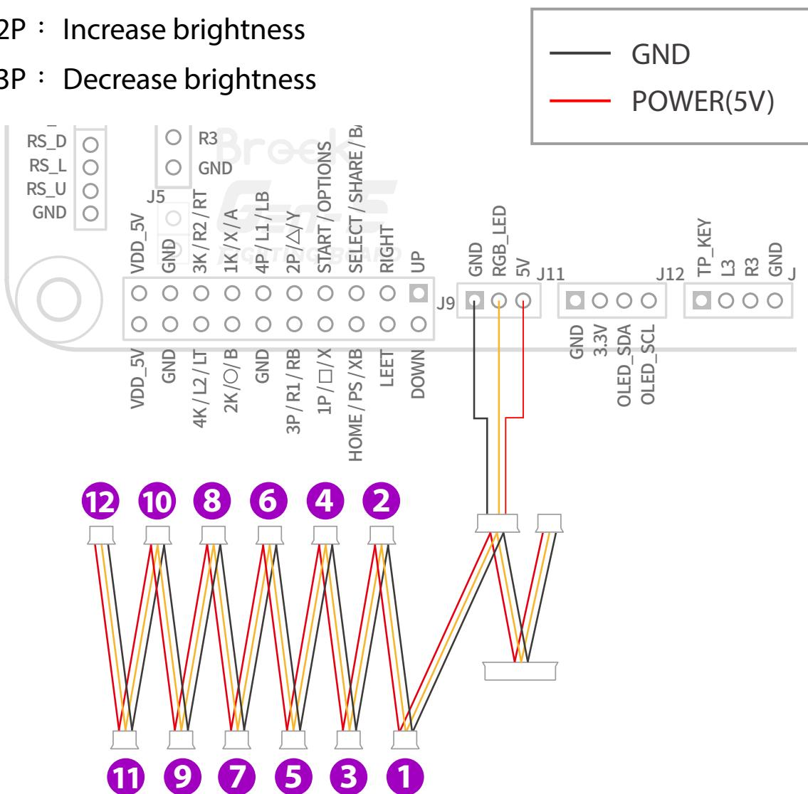
\*The order in which the RGB lights on the buttons illuminate will follow the wiring sequence. For example, the first connection will be numbered as 1, and so on.
